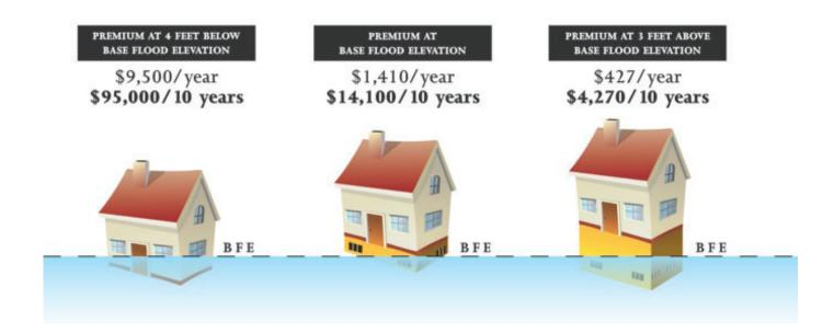
feet above the base flood level. TIP: By elevating with a freeboard of three feet or higher, flood insurance premiums can be reduced by as much as 70 percent versus rebuilding at the base flood level.
